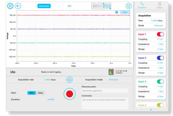
Number of InputsAcquisition RateInput RangeInput CouplingInput Impedan410 MSa/s to SSDUp to 40 VppAC or DC50 Ω / 1 MΩ
