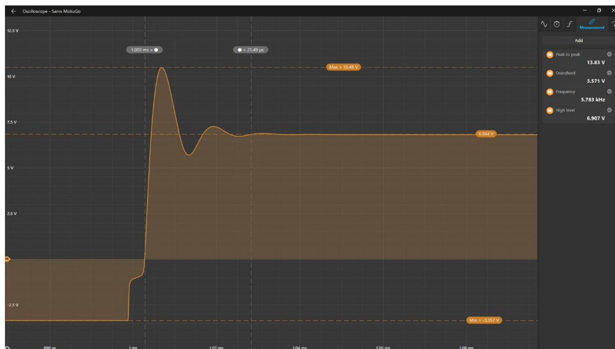
Figure 4. V_{GS} Overshoot and oscillations measurement
