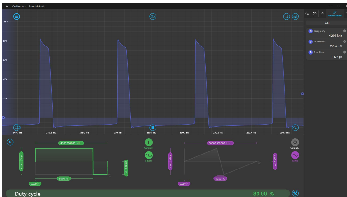
Figure 16. V_L in CC @ 4.3kHz
