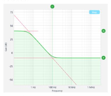
The green/purple solid curve represents the active response curve for PID Controller 1 and 2, respectively.
