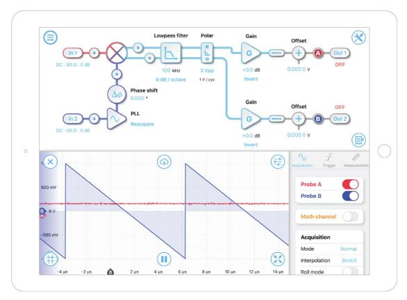
7. Tune the gain values in each arm to balance precision and measurement range.
