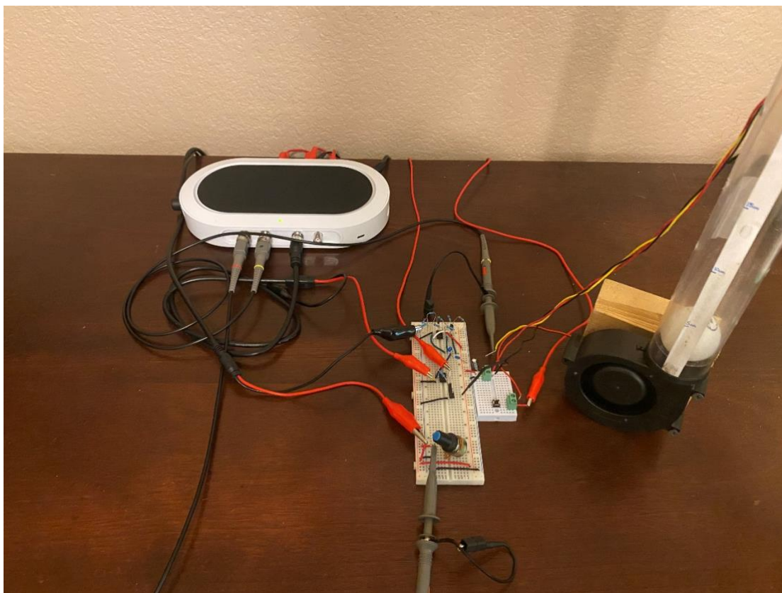
Figure 12. PID Controller Lab Setup
