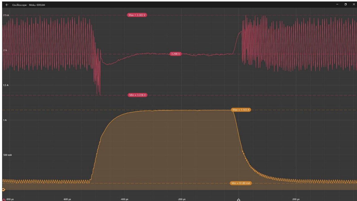
Figure 6: TPS63802 load transient response measured by Moku:Go
