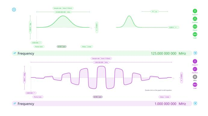
Maximum sample rate<br/>1 GSa/sOutput bandwidth<br/>300 MHzDAC resolution<br/>16-bitsIndependent triggering<br/>Burst/PulsedSupported waveforms<br/>6 predefined, segmented equations<br/>(up to 32), or custom
