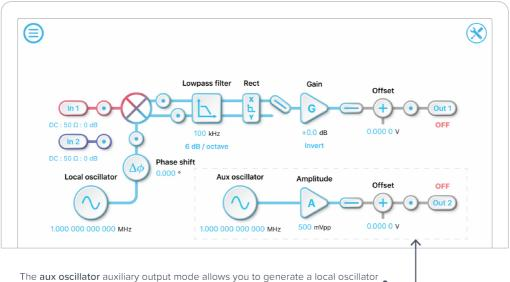
The **aux oscillator** auxiliary output mode allows you to generate a local oscillator signal with independent frequency, amplitude, and vertical offset control
